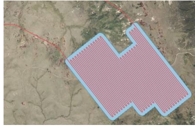
Flight Path processed into a polygon using a buffer and union tool so there are no gaps when an area is fully enclosed
