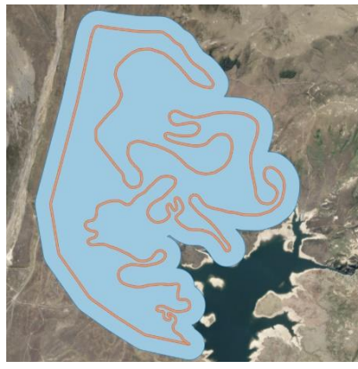
Flight Path processed into a polygon using a buffer and union tool so there are no gaps when an area is fully enclosed
